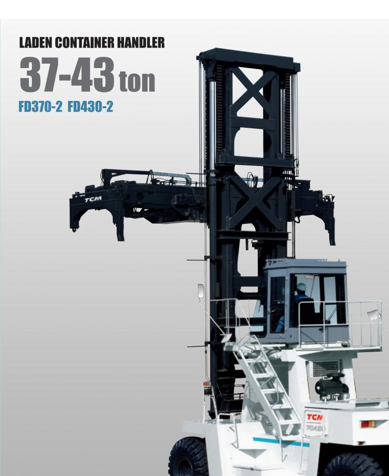
Versatile Trucks, equipped with the new type of Spreader-being capable to stack up to five containers.
