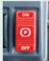
Easy to apply parking brake electronically. In addition, the electronic brake is automatically switched on when the engine halts, avoiding negligent braking when the vehicle stops.
